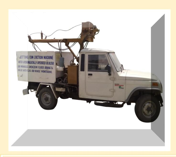
JETTING CUM SUCTION MACHIONE WITH HYDRAULICALLY OPERATED MANHOLE DESILTER WITH RODDING MACHINE HAVING WORK-STATION & TWO-WAY AUDIO-VISUAL COMMUNICATIVE CAMERA WITH MANHOLE HOLDER
